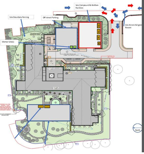
The site will be accessed from Dundee Road (A85) - as shown left. CCG's site compound will be positioned adjacent to the road on the northern boundary of the site with temporary accommodation also located towards the southern boundary as shown on the plan. Material laydown will be contained within the site boundary to minimise the impact of works at street-level.
